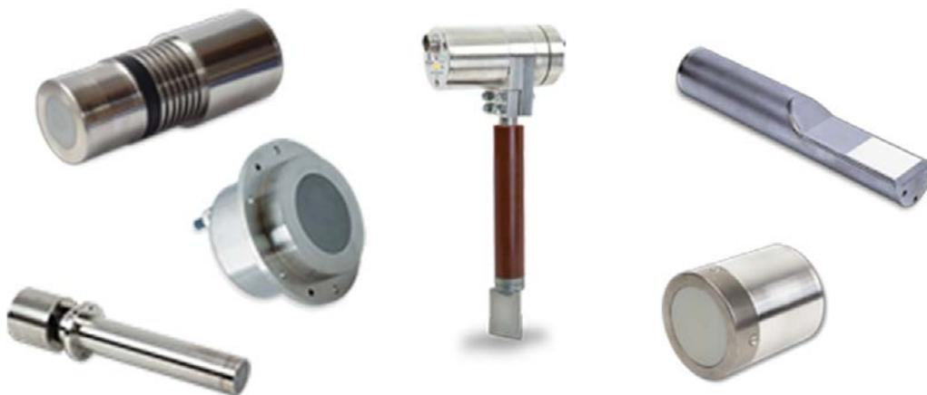
Hydronix Microwave Moisture sensors use high speed digital signal processing filters and advanced measurement techniques. This gives a signal which is linear with the change in moisture in the material being measured. The sensor must be installed into a material flow and will then give an online output of the moisture change in the material.
