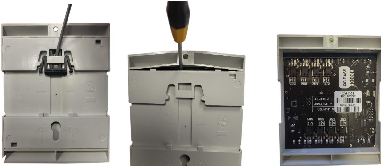
2. Set jumpers to **Current** outputs. The channel with current output must have shorted jumpers marked as current "I"
