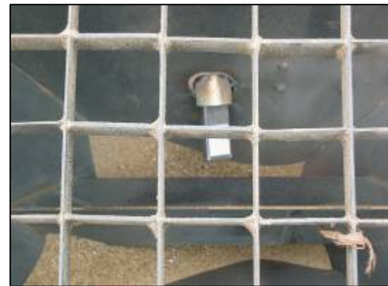
4 Ensure a good flow of material. Here a mesh is fitted for sensor protection
