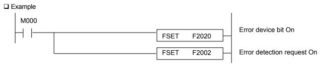
•If any trouble occurs, CPU is in error status and operation halts. At this moment, F2020 and F2002 flags are off (error LED switches on and off every second.)
