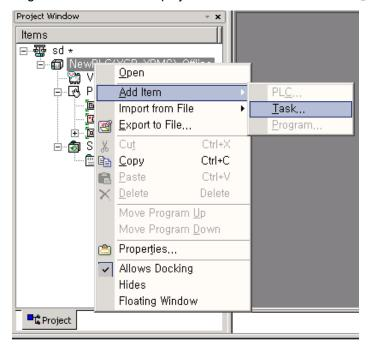
• The screen of Task setting is shown. Click Initialization in Execution condition and make a Task name.
