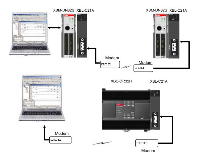
(4) 1:1 communication of an external device (monitoring unit) with main unit using a built-in RS-232C/485 port.
