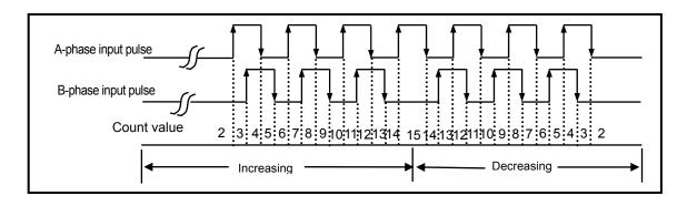
3) CW(Clockwise)/CCW(Counter Clockwise) operation mode
