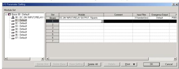
Clicking "Details" in "Slot Position" shows the following window to set filter and emergency output.
