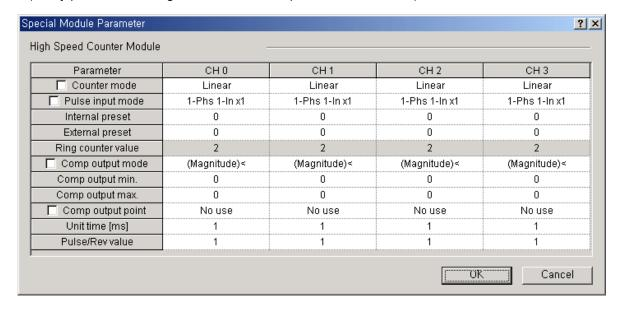
C) Turn 'ON' the high-speed counter Enable signal (CH0:K2600) in the program.
