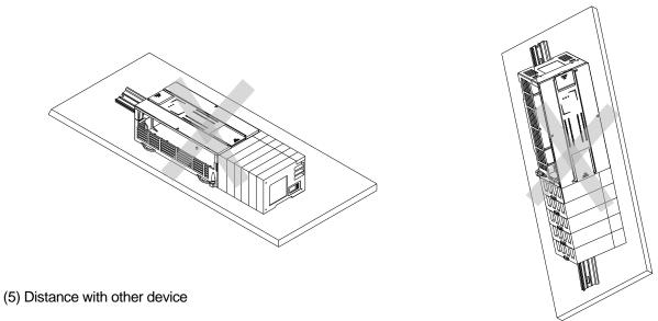
To avoid radiation noise or heat, keep the distance between PLC and device (connector and relay) as far as the following figure.
