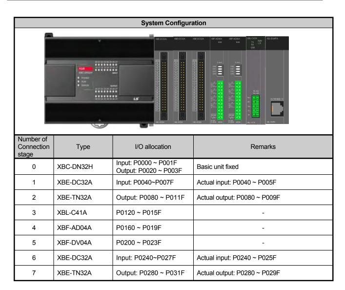
In case of using monitor function of XG5000, I/O allocation information is displayed.
