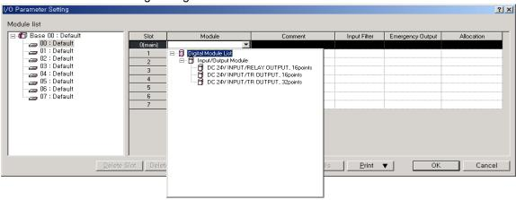
Clicking <code>"Module\_"</code> in <code>"Slot Position\_"</code> indicates a list of modules, in which you may set I/O corresponding to the actual system. Then, the following window is displayed.
