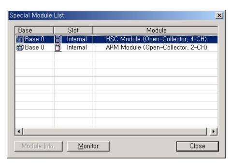
B) Clicking Monitor shows monitor and test window of high-speed counter.
