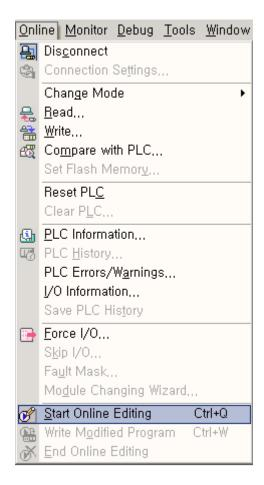
3) It turns to program modification mode during run when the program background is changed.
