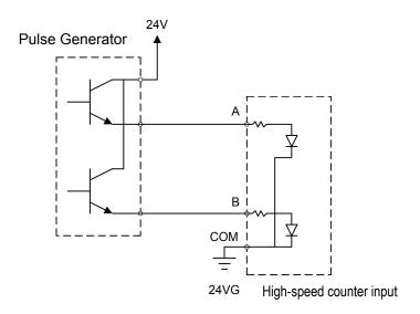
2) In case of pulse generator is open collector type
