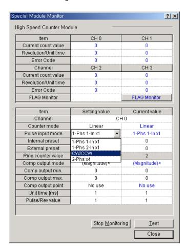
D) Clicking <code>FLAG</code> Monitor <code>shows</code> the monitor of each flag in high-speed counter, in which you may direct operation commands by flags (clicking commands reverse turn).
