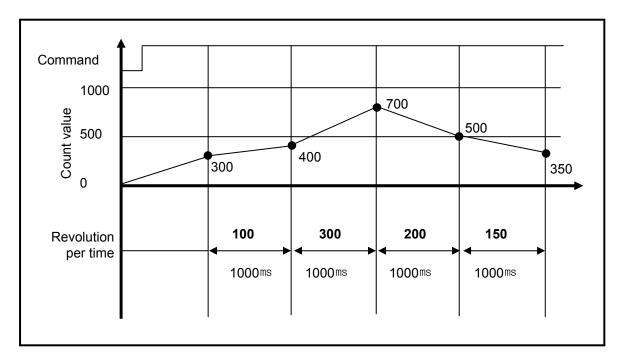
F) In order to indicate revolution per minute (RPM), the program is as shown below. In case of DMUL operation, RPM value is saved 64 bit in D100~D103. If operated RPM value is used, it can use to Word or Dword type according to system (case of RPM value is small number).
