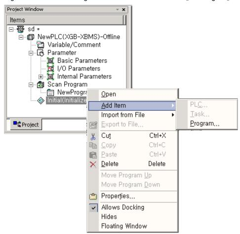
• Make initializing program. In initializing program, INIT\_DONE instruction must be made. If not, Scan program is not executed.
