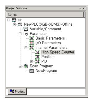
B) Selecting high-speed counter opens a window to set high-speed counter parameters as follows. For details regarding each parameter setting, refer to 8.1~8.3. (Every parameter settings are saved in the special K device area.)
