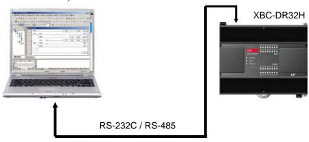
(2) 1:1 communication with main unit using a built-in RS-485 port (In case of built-in RS-232C, it is for connecting to HMI device.)
