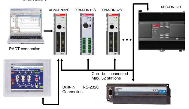
(2) Using RS-485 built-in function/expansion Cnet I/F module can be connect for up to 32 stations.
