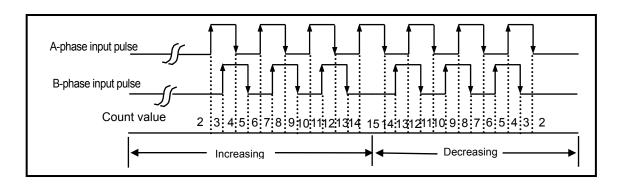
3) CW(Clockwise)/CCW(Counter Clockw'ise) operation mode
