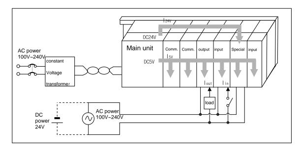
(e) Input average power consumption of input module (power consumption of simultaneous On point)
