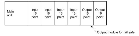
Equip output module for fail safe to last slot of system.
