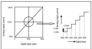
In current output, digital amount 0 exchanges to 4mA, and 4,000 does 20mA. Analog amount of digital input 1 equals to 6.25  $\mu$ A.
