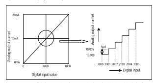
In current output, digital amount 0 exchanges to 0mA, and 4,000 does 20mA. Analog amount of digital input 1 equals to 5  $\mu$ A.
