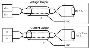
\*1 : Be sure to use two-core twisted shield wire.
